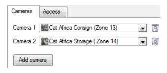
Adding a camera to an object will mean that, whenever there is an event on that object, the recording from that camera will be related to the time and date of the object event, in the Integration database.
