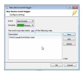
For example, within the any device event option, choose the type of device Event that will be a trigger. Choose from the drop-down menu. The ACT device offers Alarm, Door, General, and Reader Events.
