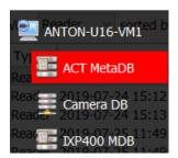
When the Database Tab 3.2 opens, select the relevant integration database from the database panel that opens on the left-hand side. The databases are ordered under the NVRs that they are attached to. See below for the ACT database.
