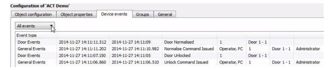
The Device Events tab, lists real time events happening on this device. It is an excellent way for installers to see that the integration is functioning, and to monitor the live events happening on site.
